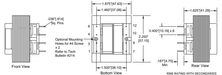
SECONDARY WINDINGS ARE DESIGNED TO BE USED AS ONE SECONDARY WINDING WITH EITHER PARALLEL OR SERIES CONNECTIONS ONLY!
